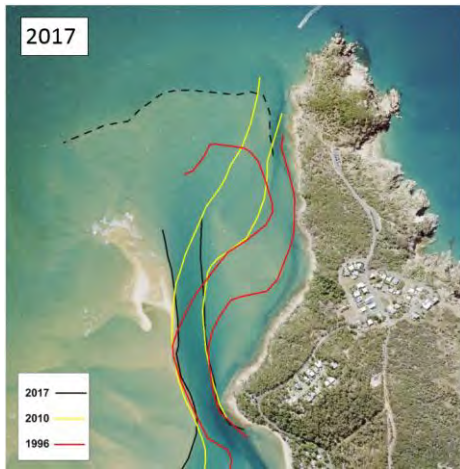
Figure 3-5 Recent Channel Locations shown on 2017 Photo
