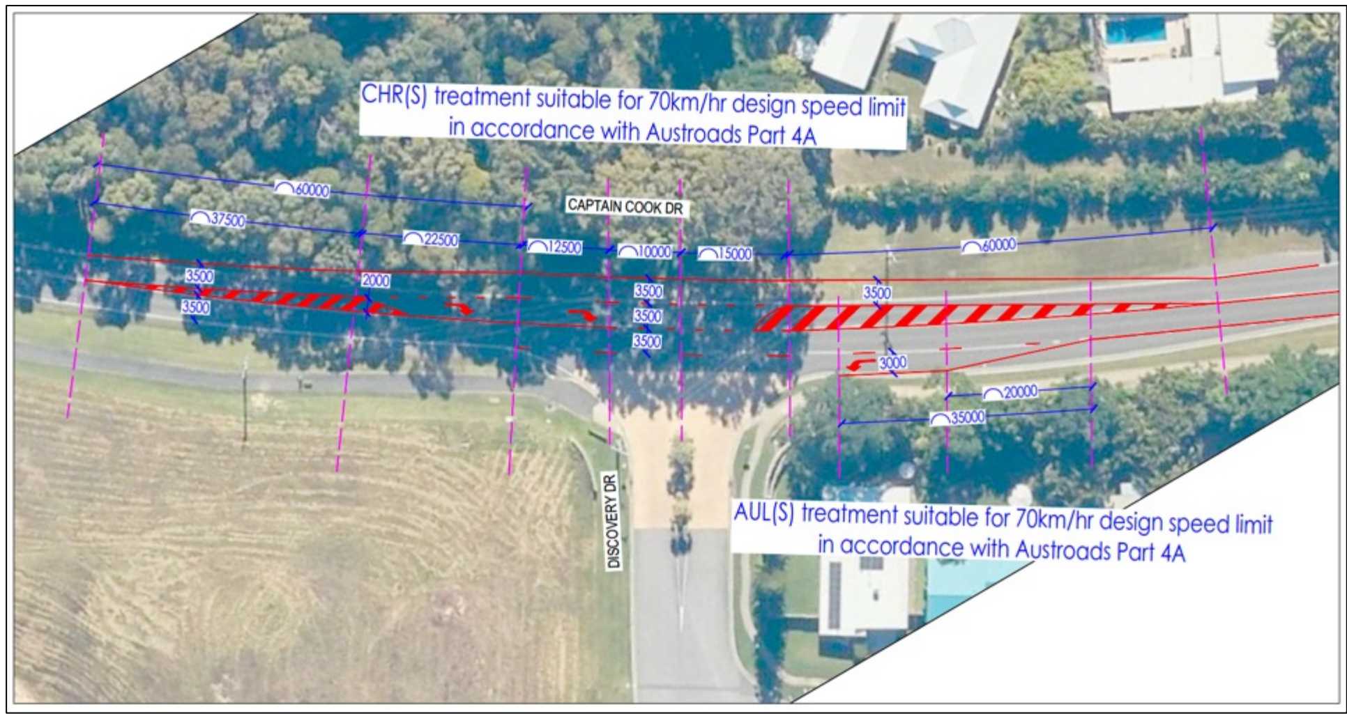
FIGURE 5.4 – CONCEPT LAYOUT OF REQUIRED UPGRADE TO CAPTAIN COOK DR / DISCOVERY DR INTERSECTION FOR FUTURE STAGES OF DEVELOPMENT
