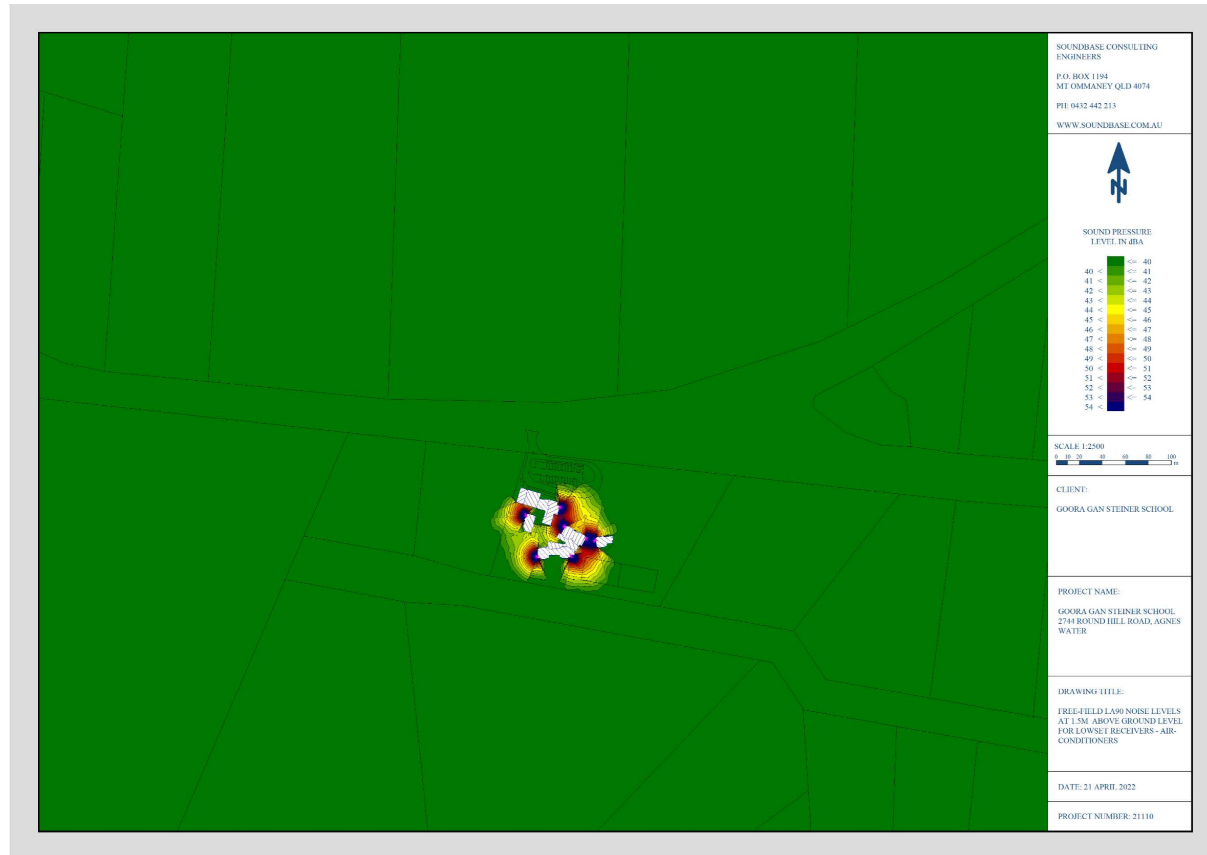
Figure 7: LA90 noise emissions from the air-conditioning condensers for comparison against background creep limits
