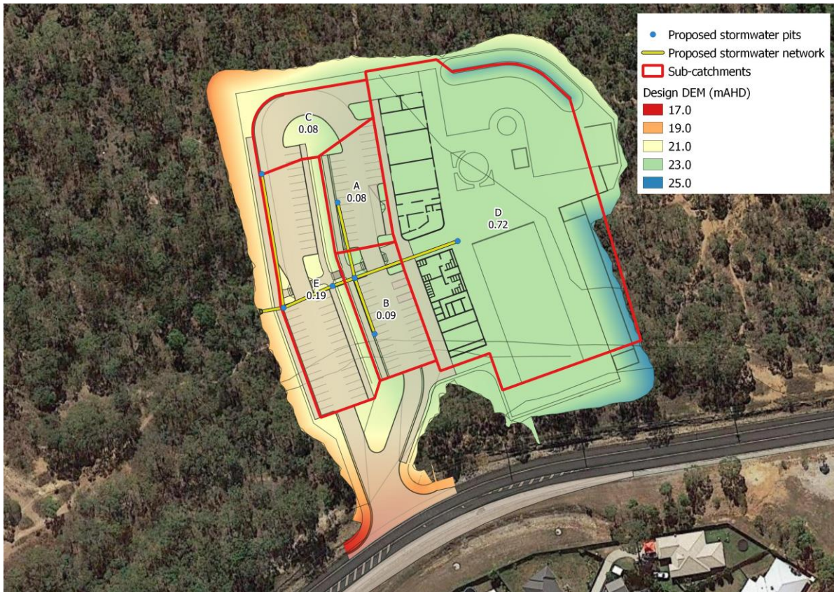
Figure 2.1 Proposed stormwater network and corresponding sub-catchments with their area in hectares
