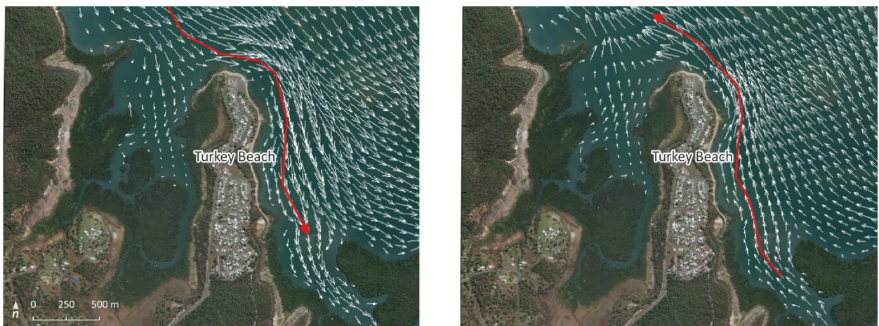
Figure 10. Modelled tidal patterns around Turkey Beach showing peak flood-tide (Left) and ebb-tide (Right) (white arrows) and overall dominant direction (red arrows)
