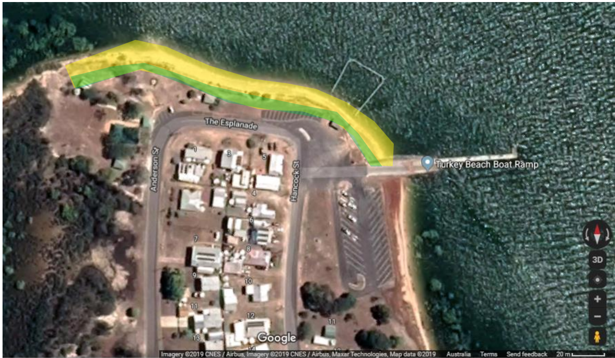
Figure 32. SEMP Part B – northern point – beach nourishment and revegetation – indicative nourishment area (4,000 - 5,000 m 2 ) and vegetation area (2,000m 2 )
