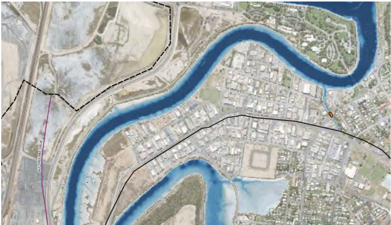
Figure 6-3 1% AEP Peak Depth in Lower Region of Auckland Creek
