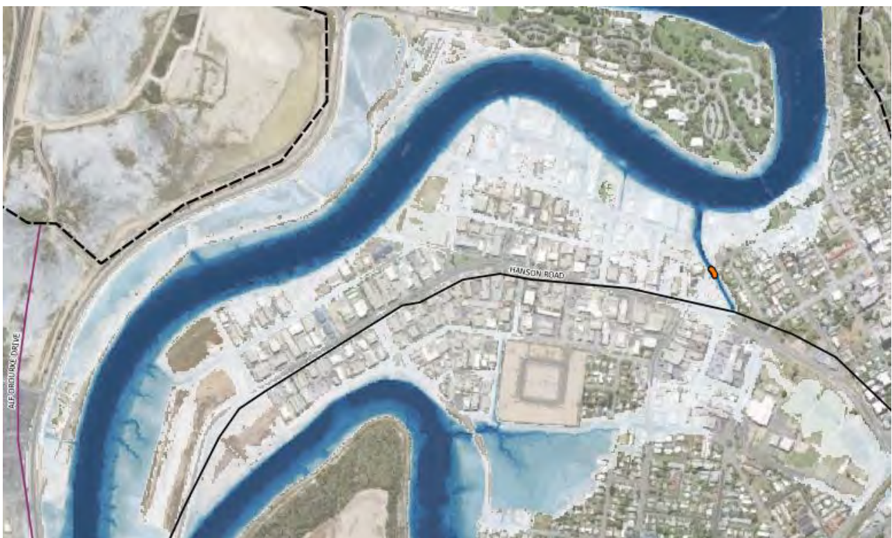
Figure 6-4 1% AEP Peak Storm Surge Depth in Lower Region of Auckland Creek
