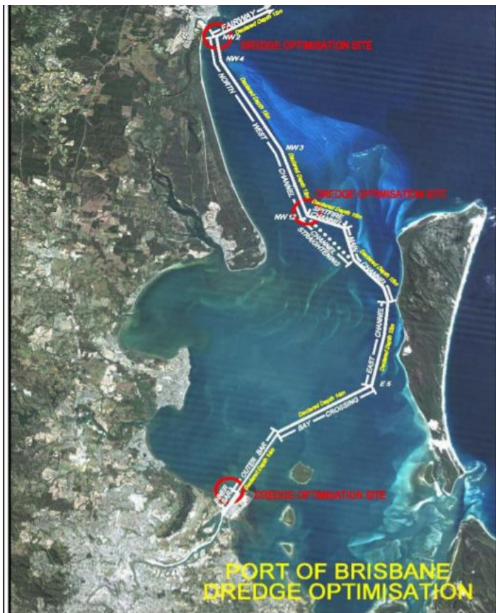
Figure 3.5. Dredging Path to Enable Larger Container Ships
