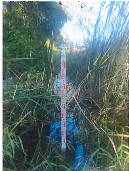
P06 Photo same position with survey staff pushed by hand into the mat 1 metre below water
