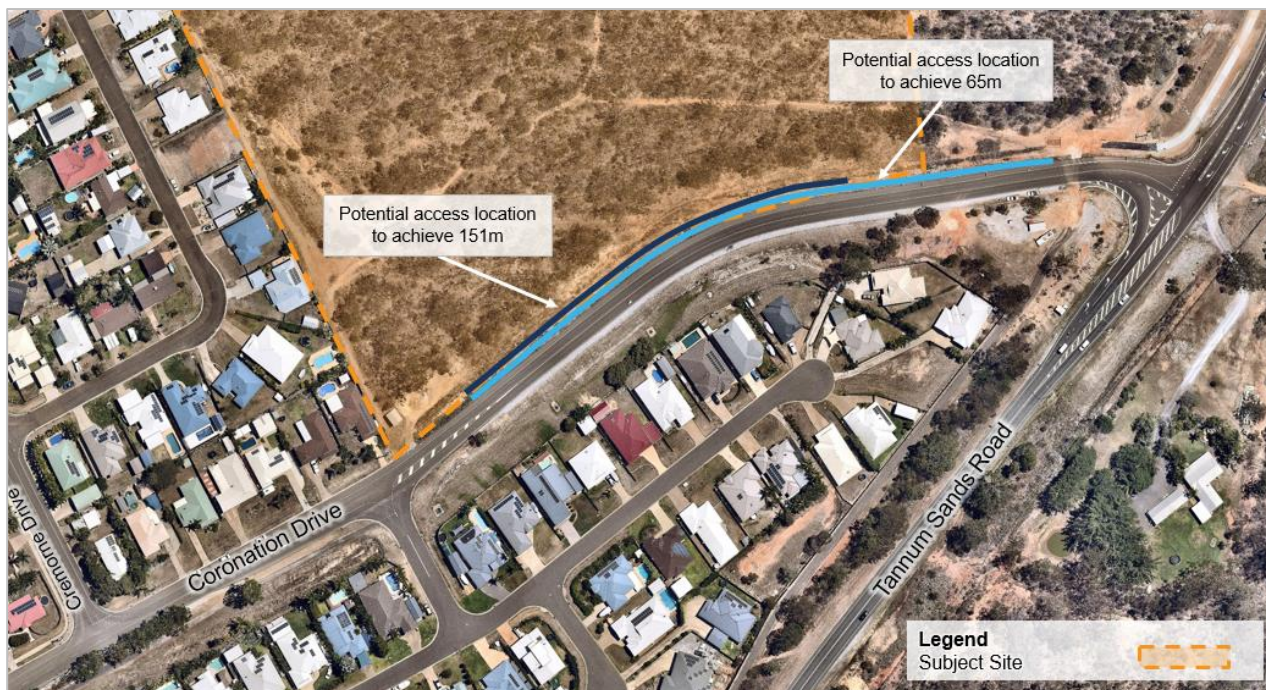
Figure 6-5 Potential access location to achieve sight distance Note the site boundary is indicative only. Source: Nearmap.
