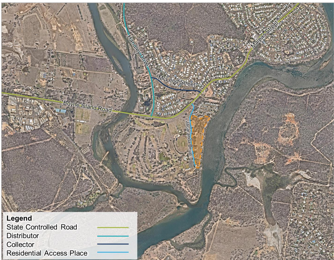
Figure 6-1 Local site context and road hierarchy Note the site boundary is indicative only. Source: Nearmap.
