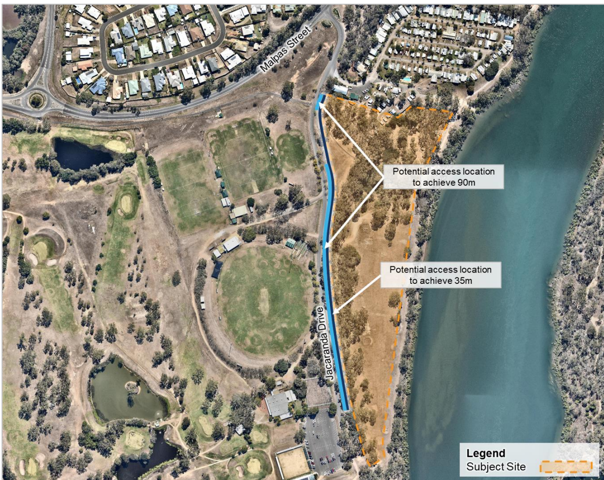
Figure 6-5 Potential access location to achieve sight distance Note the site boundary is indicative only. Source: Nearmap.
