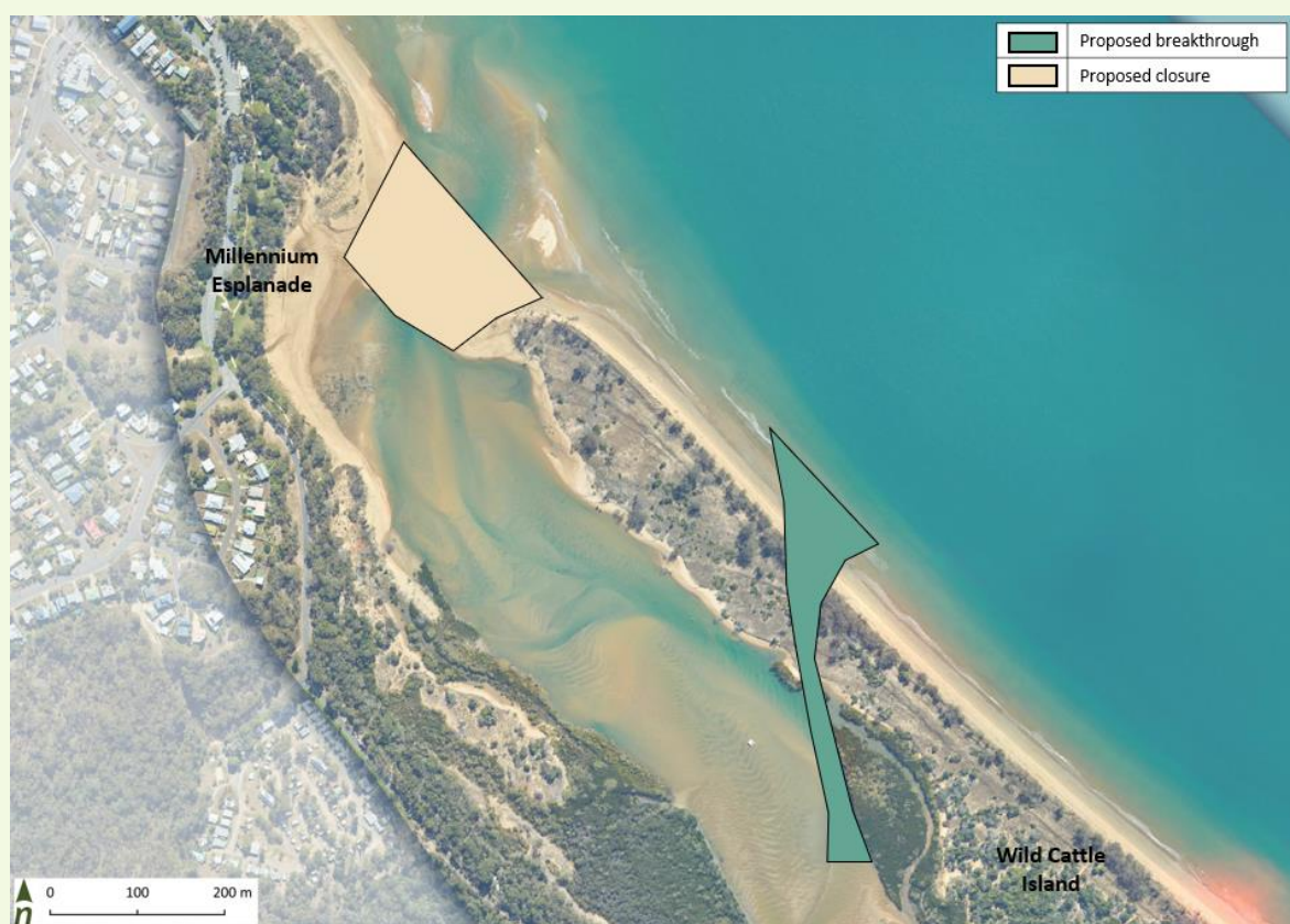
Figure 35. Millenium Esplanade – Option 3 – Artificial breakthrough
