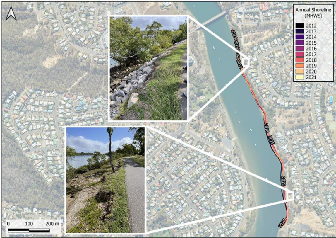
Figure 7-4: CoastSat analysis shoreline positions along the Turtle Way over a 9-year period
