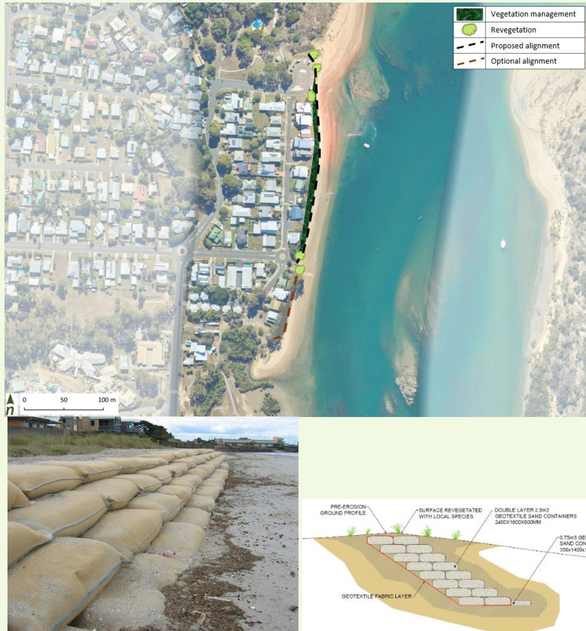
Figure 26. Island Esplanade foreshore – Option 2 – Concept plan and illustration of GSC seawall.
