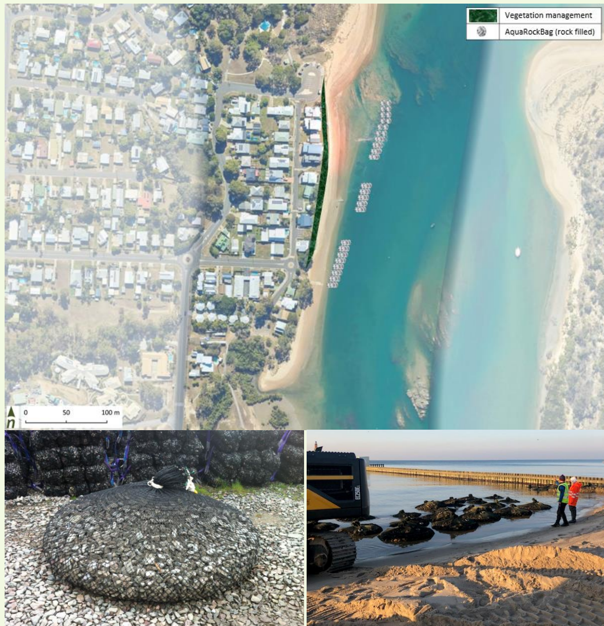
Figure 29. Island Esplanade foreshore – Option 5 – Concept plan of AquaRock Bags structure alignment. (Bottom) Photos sourced from Gabion Cages and Baskets.
